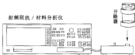
图5 “带内导体开路器”阻抗测量值的校准
